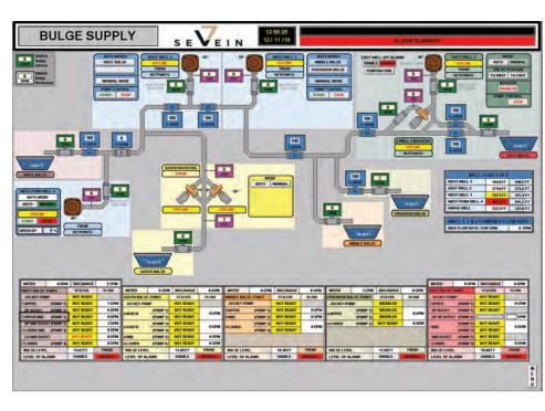
A command-and-control nerve center called SCADA (Supervisory Control and Data Acquisition) provides real-time observation and control over millions of gallons of water coursing through 10 miles of arterial mainlines.
