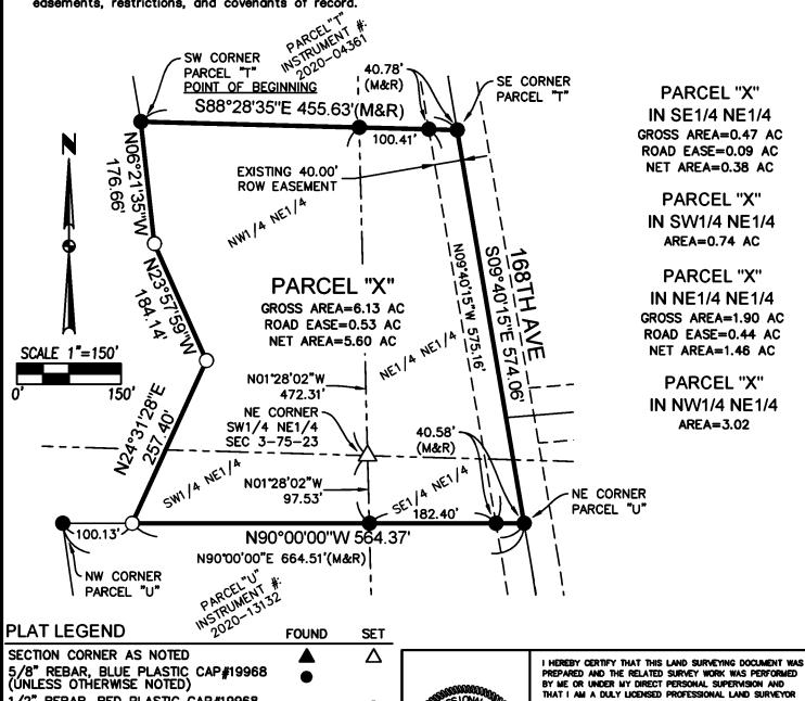
/2" REBAR, RED PLASTIC CAP#19968 UNLESS OTHERWISE NOTED) 0 MEASURED BEARING & DISTANCE (M) RECORDED BEARING & DISTANCE (R) DEEDED BEARING & DISTANCE (D) CENTERLINE SECTION LINE EASEMENT LINE
