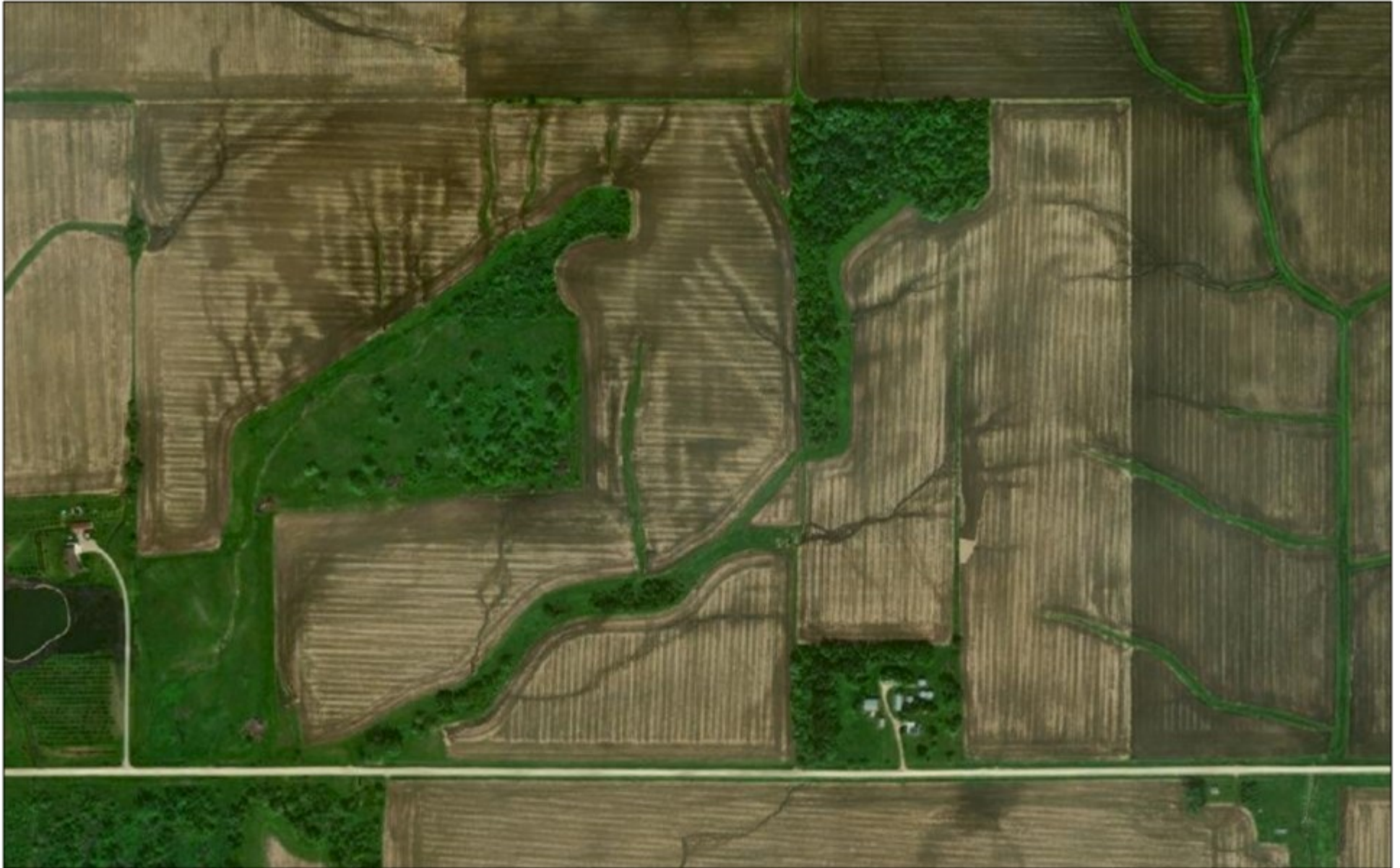
Aerial image showing approximate tile line locations
